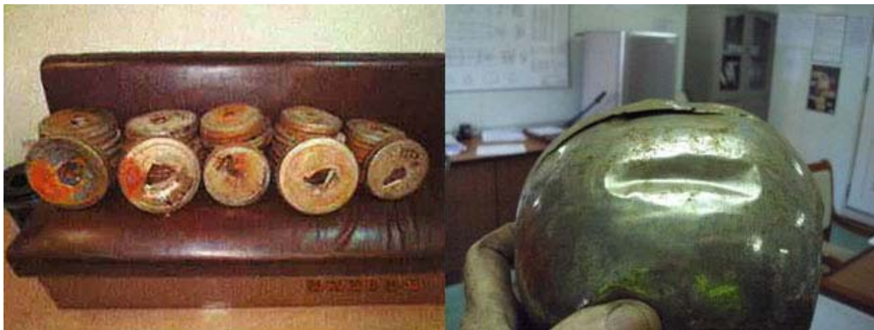
Damaged floating devices in air-pipes heads subjected to continuous overflow
