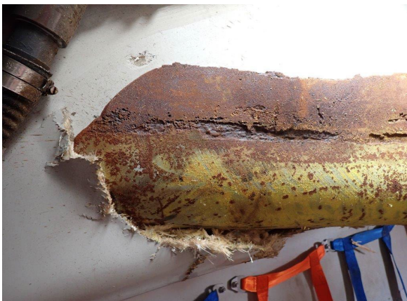
Figure 2: Severely corroded remnants of compressed air cylinder shell. Note the distinct line of deep pitting.
