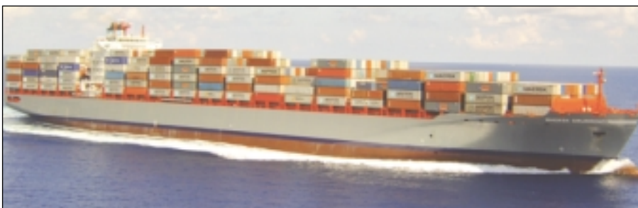
Pictured is the 5,041 teu-capacity, Liberian-flag panamax containership "Maersk Drummond", which was built in 2006 by Hyundai Heavy Industries, South Korea
