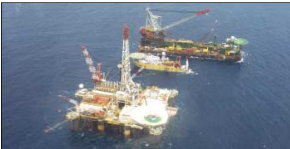
The "Sedco 700," which flies the Liberian flag, is a semi-submersible drilling unit capable of operating in harsh environments and water depths of up to 3,600 feet. Built at the Levingston Shipyard in Texas, it is classed by ABS and has accommodation on board for 120 people.
